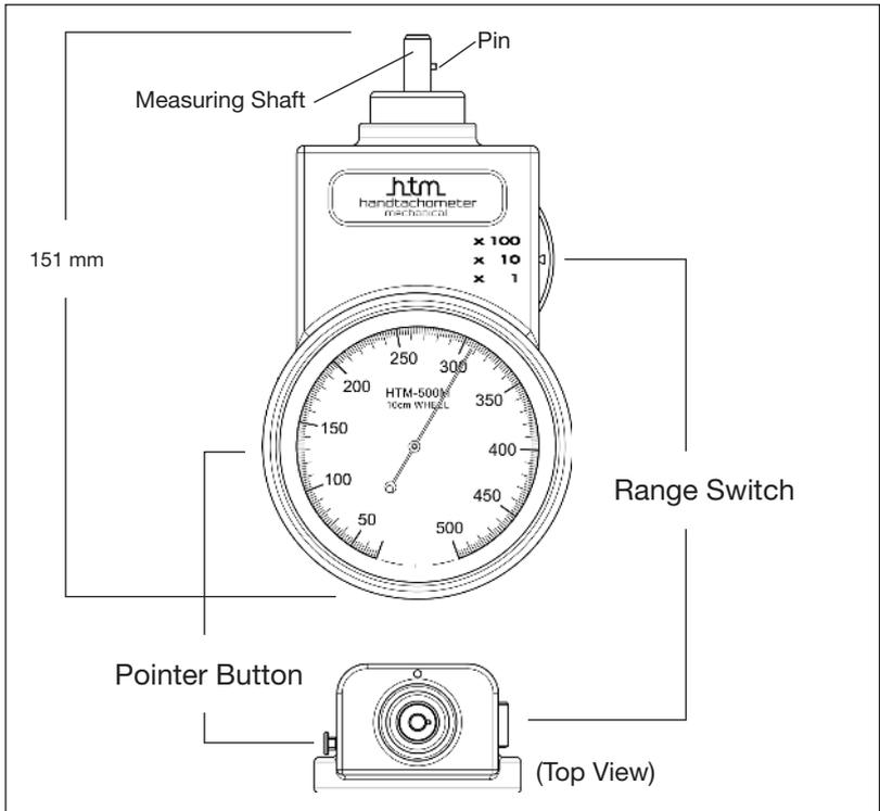
1. Slide the **Red Range Switch** to select a multiplier for your application. If the range is unknown, start at "x100" and adjust to lower range as needed. When properly set, the needle will register a value between Min. and Max. on the dial.
